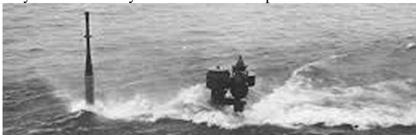
A U.S. Navy submarine with periscope and snorkel in use.
