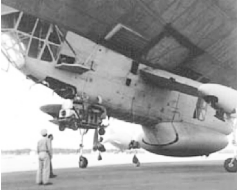
Loading an Auxiliary Power Unit on to the weapons rack of our Nan-ship.
